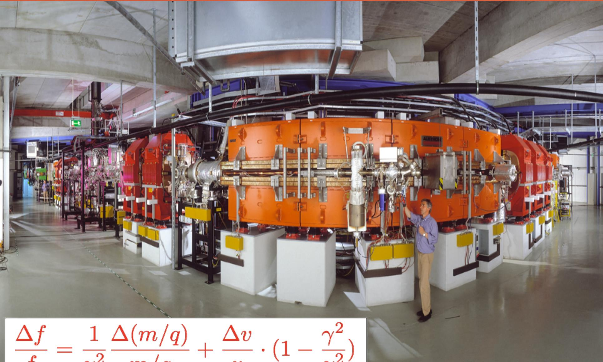
$$\frac{\Delta f}{f} = \frac{1}{\gamma_t^2} \frac{\Delta(m/q)}{m/q} + \frac{\Delta v}{v} \cdot \left(1 - \frac{\gamma^2}{\gamma_t^2}\right)$$
