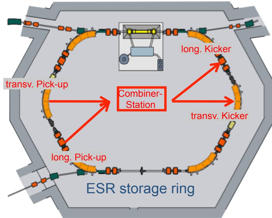
Stochastic cooling is in particular efficient for hot ion beams
