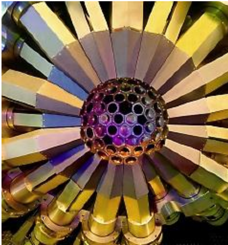
up to 110 Compton-Suppressed Ge detectors
