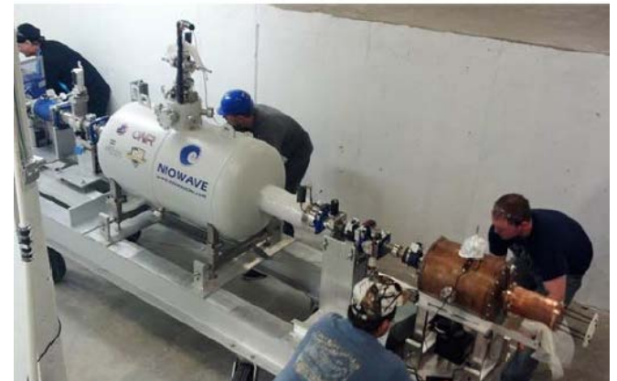
Figure 2. A compact superconducting accelerator used for radioisotope production
